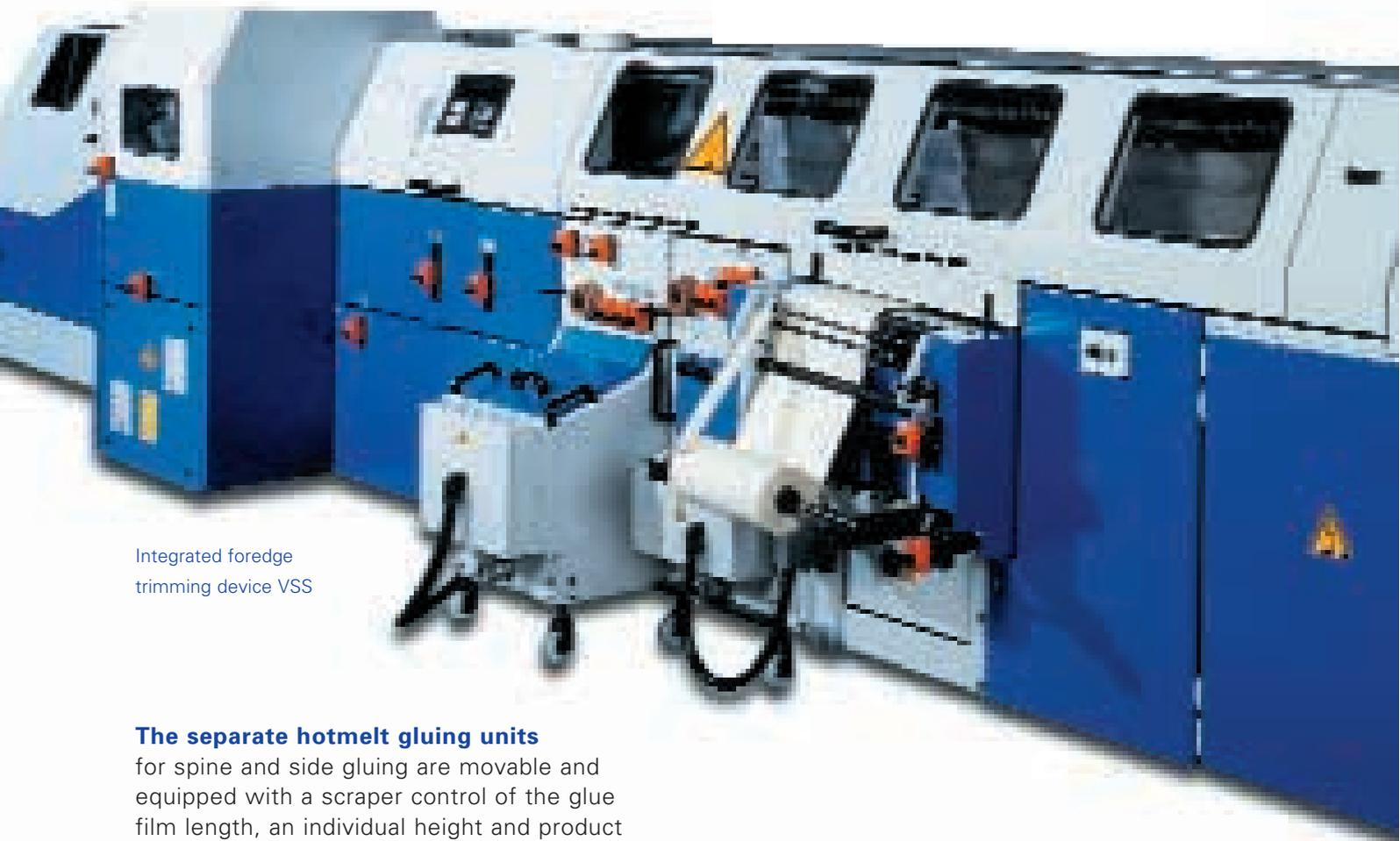
Integrated fore-edge trimming device VSS
